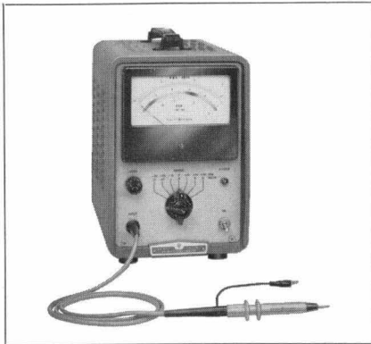
Fig. 3. -hp- Model 411A RF Millivoltmeter. Probe is arranged to accommodate many measurement conditions since basic probe tip with flange-operated alligator jaws as shown is removable; probe can then use various specially-designed accessories such as rf fittings for measurements in coax cables.
