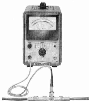
Fig. 1. New -hp- Model 411A RF Millivoltmeter makes sensitive voltage measurements to 1 kilomegacycle with -hp- coax tee (foreground) and gives useful voltage indications to above 3 kilomegacycles. If desired, sweep-frequency voltage measurements can be recorded, as in Fig. 2, using dc output provided by 411A.
